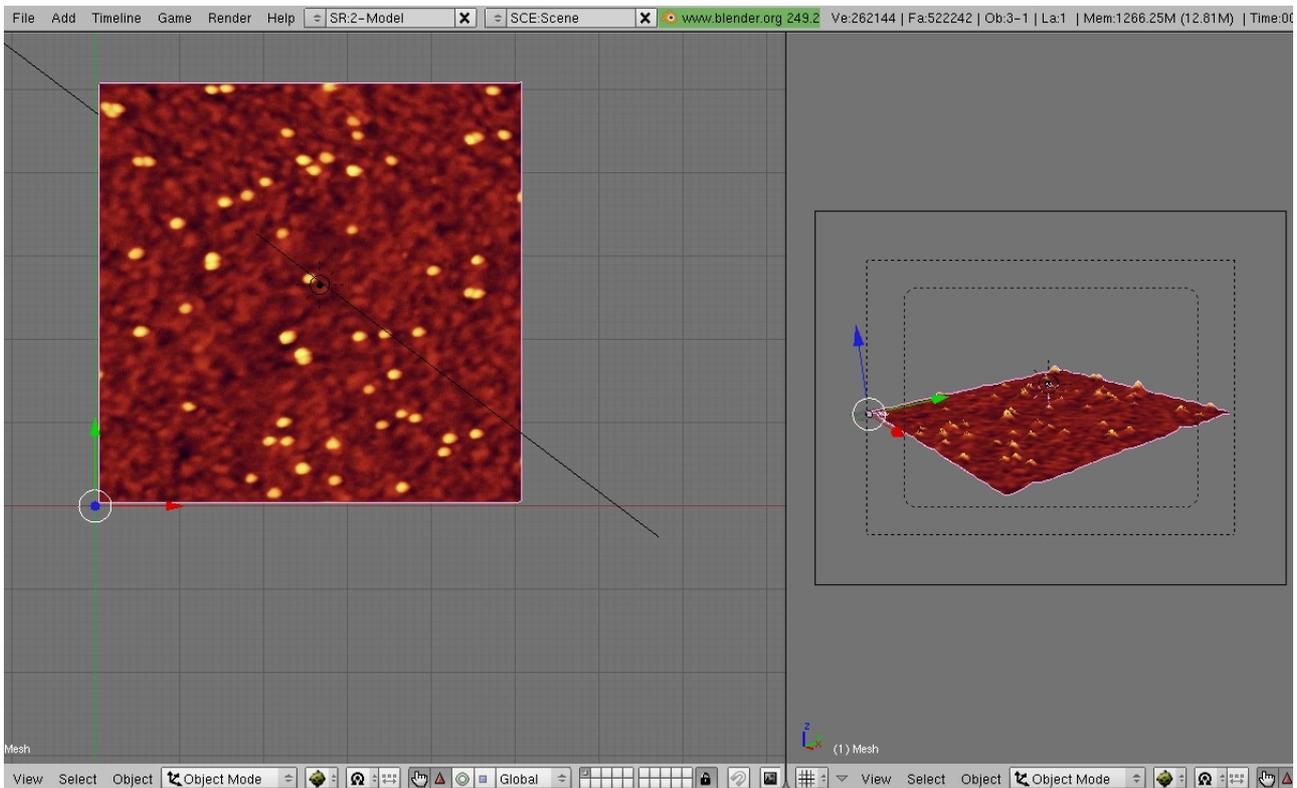
The left window show the top view of the Mesh (number 7). The lamp is positioned in the middle over the Mesh. The dashed line indicates the direction of the camera view. The right window show the view through the camera (number 0).
