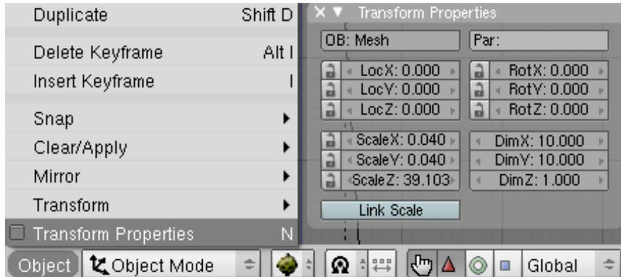
With DimZ you can alter the Mesh in z-direction. The larger DimZ the larger become expansion in z-direction. If DimZ is “0” your Mesh is in 2D.
