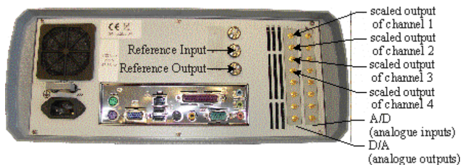
Figure 11: Rear-Panel of the eLockIn (picture might vary from current revisions). The ground connector above the power supply allows to separate the protective ground from the housing and thus increase the resistance between them to 1 MOhm.
