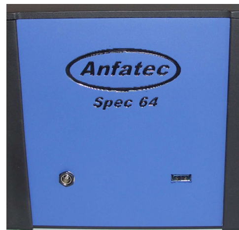
• Figure 2: Power Supply for 12 V dc (left) and USB-Connector (right)
