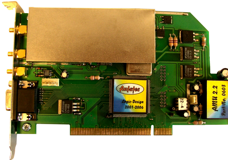
Figure 6: Photograph of the LockIn board and description of the location of the single parts.
